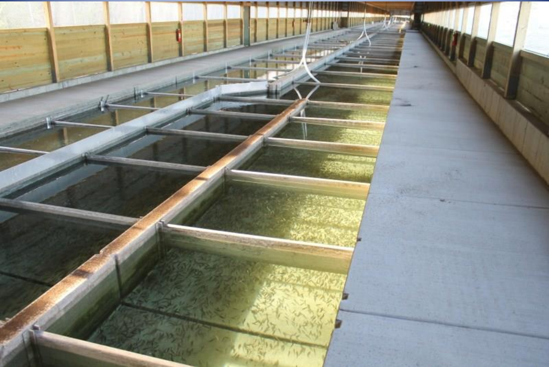
Great Lakes Steelhead-RBT in Baffled Production Raceways with New Biosecure Raceway Enclosures
