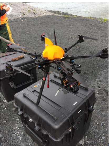
Gyrostabilized Sony Nex7 and GoPro ~20 min/fligth (LiPo batteries)
