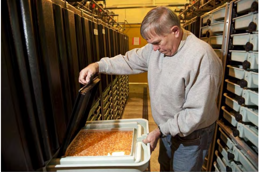
HDR's Senior Fisheries Biologist Tom Johnson inspects salmon eggs in vertical flow incubator in Coldwater Production Building
